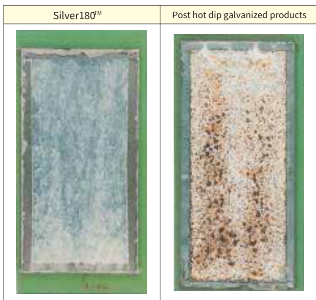
Appearances after 450 hours of sulfur dioxide test
